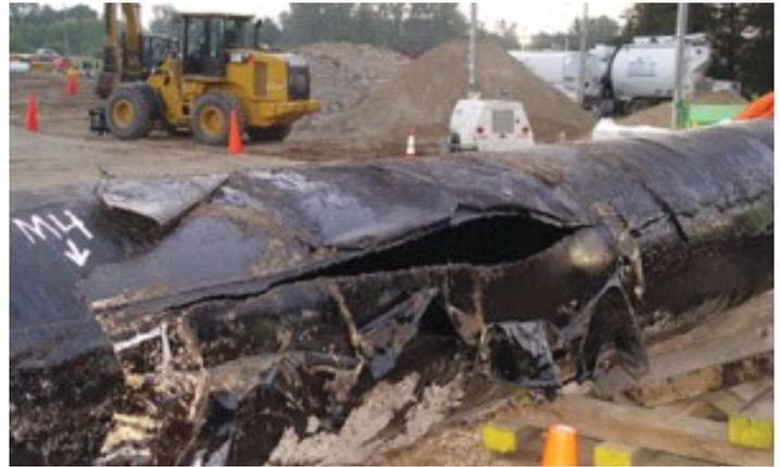
Section of ruptured pipe from Kalamazoo River spill in Michigan. Rupture length is approx 6 ft 5 inches and is 4 1/2 inches wide at the widest location. (photo by National Transportation Safety Board)
